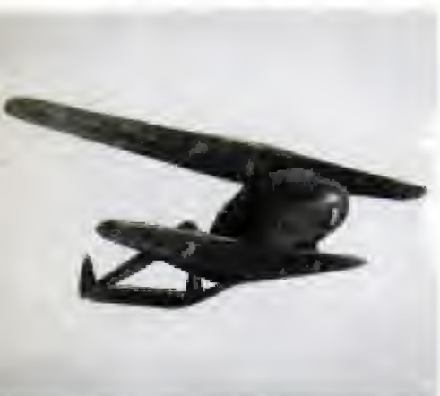
Rotor of Herrick model becomes the main wing for forward flight
